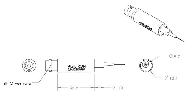
dimensions tolerance to be +/-0.2mm
